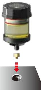
Remove the protector from the output thread and use appropriate adapters to install on the lube point.
