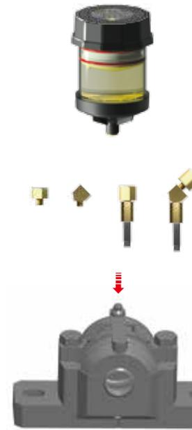
When there are space restrictions of the application that will not allow a direct straight mount, use a 45° or 90° fitting for Direct Angle Mount.
